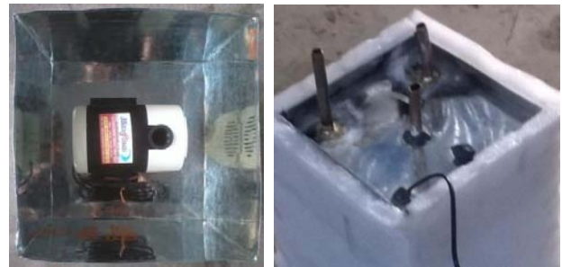
Fig. 9: Pump with Supply Reservoir
