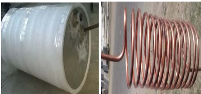
Fig. 7: Heat Exchanger with Coiled Copper Tube
